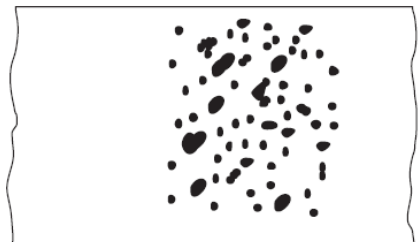
(a) Random Rounded Indications Typical concentration and size permitted in any 150 mm length of weld.
